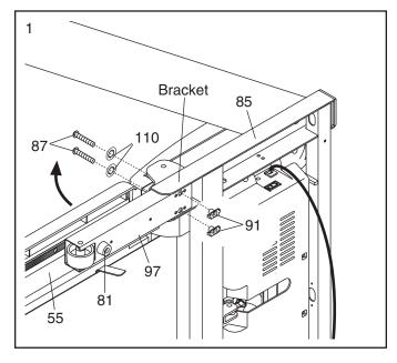
Attach two Base Pads (81) to the base of the Uprights (85) in the indicated locations with two 1" Tek Screws (82). Note: One replacement Base Pad may be included. Use the Base Pad to replace any Base Pad that becomes worn.
